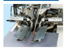
The dart stretcher clamps the end of material to smooth out the wrinkles on a garment body, thereby allowing the sewing machine to perform welting with consistency.
