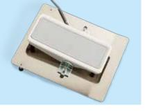
One-shot operation pedal is adopted to start the sewing machine. The sewing step is moved forward by depressing the front part of pedal, and it is moved backward by depressing the rear part of pedal.
