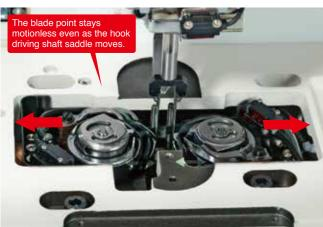
Image of adjusting the hook driving shaft saddle
