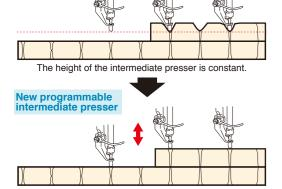
The intermediate presser goes up and comes down according to the material thickness
