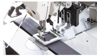
Example application: Reinforcing the stitching of seatbelts
